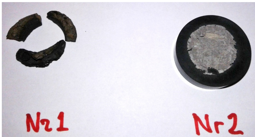
Figure 1. Samples produced by SPS from ash.
