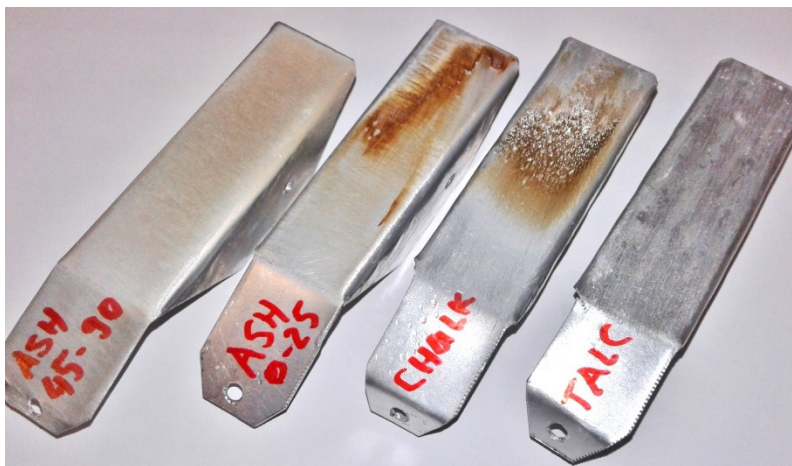
Figure 8. Results of testing with “ski” type sample. Clear formation of new surface layer is visible in case of chalk and ash.
