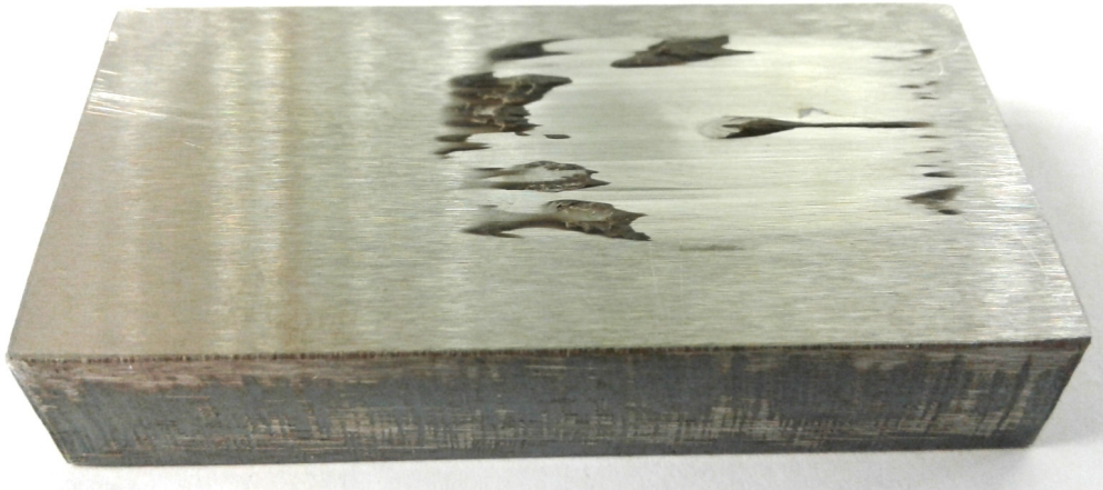
Figure 9. Hardox 400 sample after 10 minutes of abrasion by ash.
