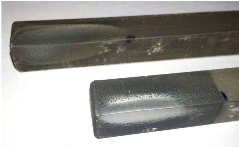
Figure 5. Typical wear scar after test with abrasive powder (not result of current test).
