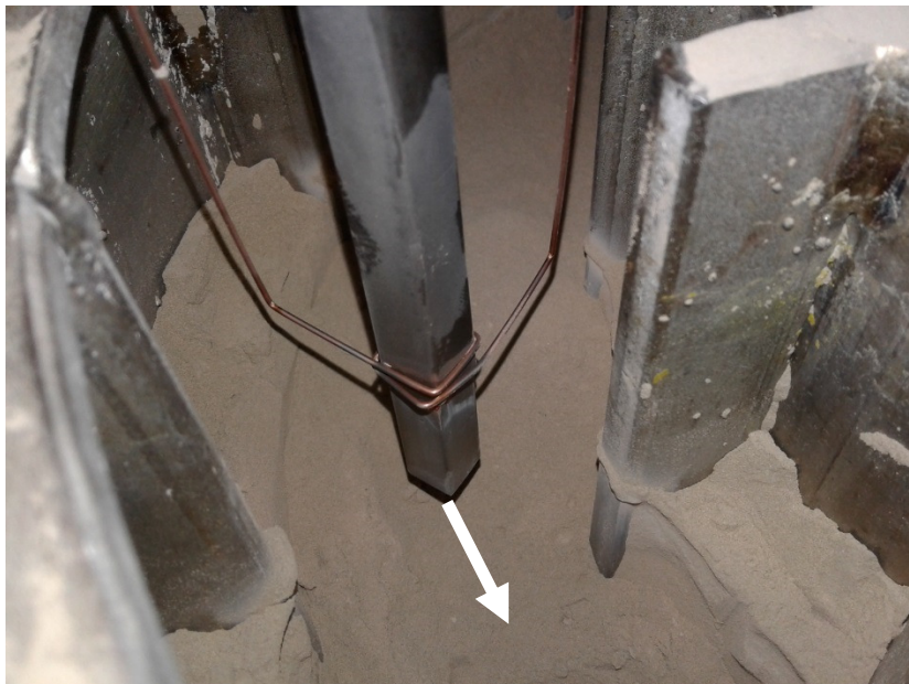
Figure 4. Sample installed into HLTS with indication of movement direction. The sample is not immersed into powder yet.
